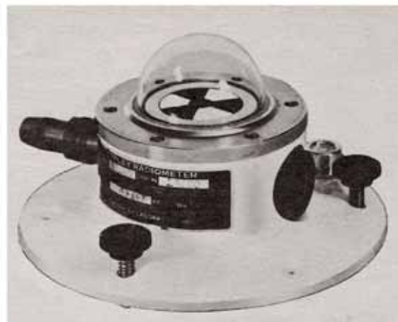
Figure 2.3.2 The Eppley Black and White Pyranometer. Courtesy Eppley Laboratories.
