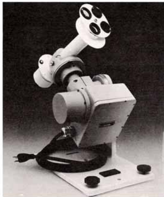
Figure 2.2.4 An Eppley Normal Incidence Pyrheliometer mounted on an altazimuth tracking unit. Courtesy Eppley Laboratories.
